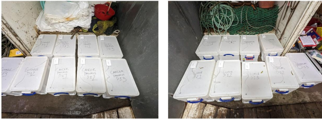
Figure 4.2 (a) The holding tank set-up within the cold store of the fishing vessel, designated for a specific species and damage index. Each holding tank was created from a 42L storage box with a battery-operated airline attached to the lid which provided continuous aeration to the ambient seawater.
