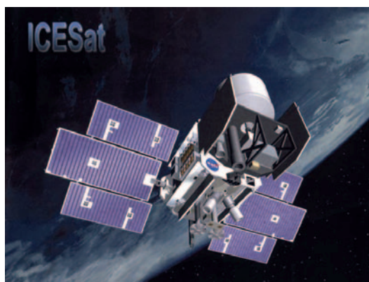
Figure 1. The ICESat laser illuminates a ground footprint of approx. 70 m extent.
