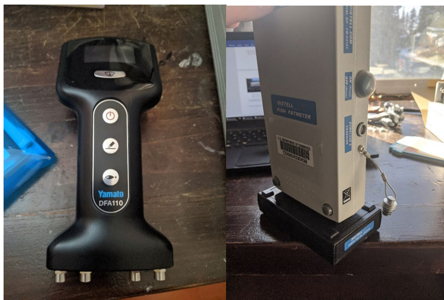
Figure 19. -- The Yamato Fish Analyzer (left) and the Distell Fatmeter (right). Both meters are easily hand-held and are placed on the fish musculature to read the index of lipid content.
