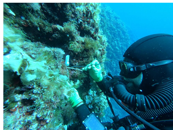
FIGURE 7 Underwater manual sensor mounting by diver.
