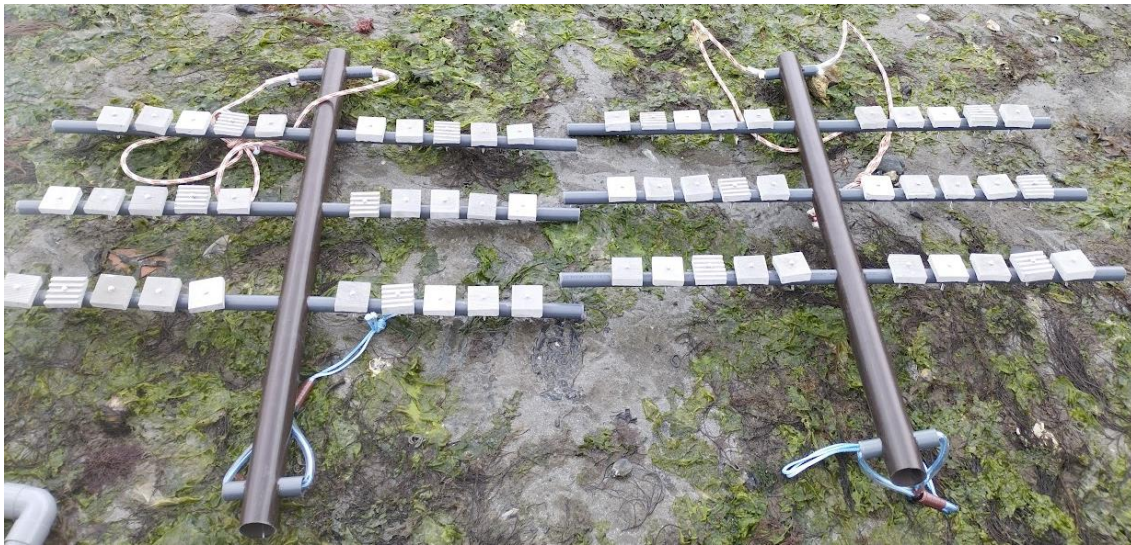
Figure 5.4: Picture of the different frames used to deploy concrete tiles in the field experiment. The top image is the parallel frame, and the bottom image is the perpendicular frames.
