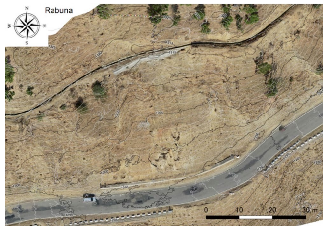
Fig. 3 Gully erosion developed on the slope after bioengineering work (Rabuna, Wangdue, photo by drone on January 11, 2024)
