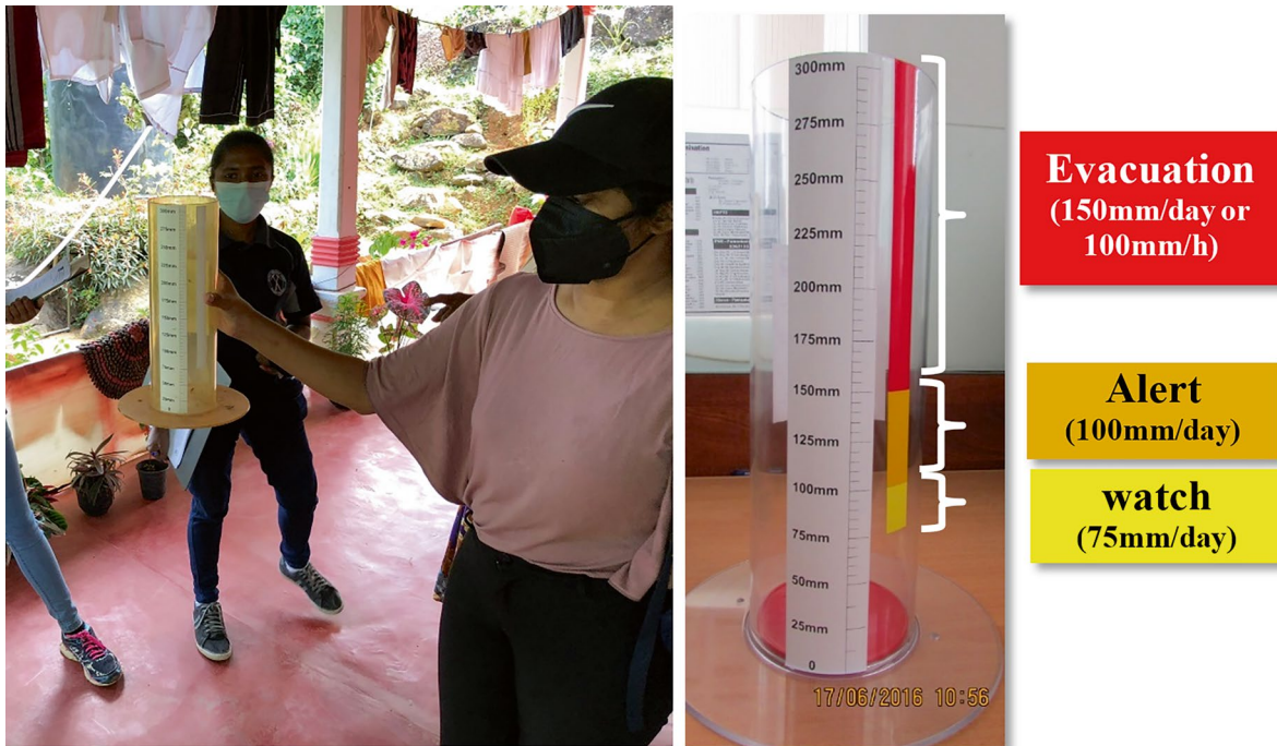
Fig. 12 Manual rain gauge with a scale on its side: The scale has the color-coded upper three levels (Yellow for 50–100 mm/day), (Orange for 100–150 mm/day), and (Red for 150 mm and beyond). The photo on the left was taken at 7.1620N, 80.436E, on January 9, 2023
