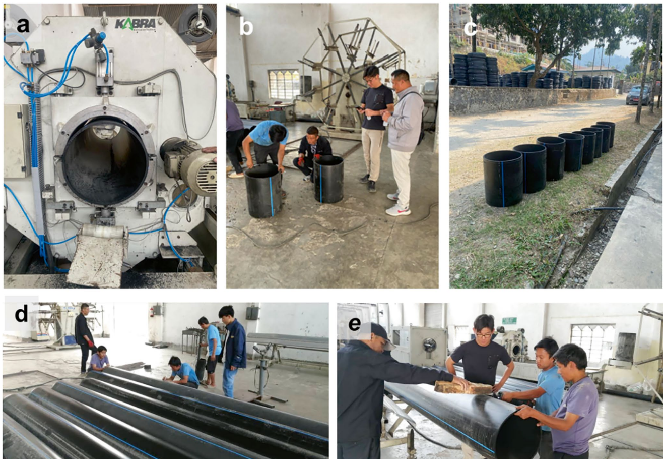
Fig. 38 Preparation of vegetation pots ((a) Cutting machine, (b, c) vegetation pots, (d, e) HDPE tube)
