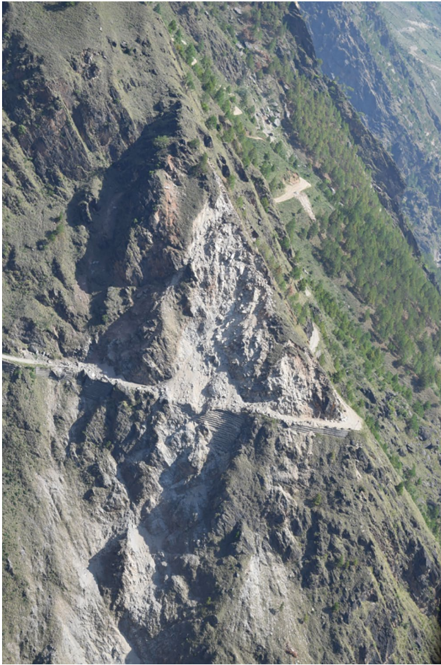
Fig. 64 Typical landslides triggered by the 2015 Gorkha Earthquake along the Nuwakot-Dhunchhe-Rasuwagadi Road
