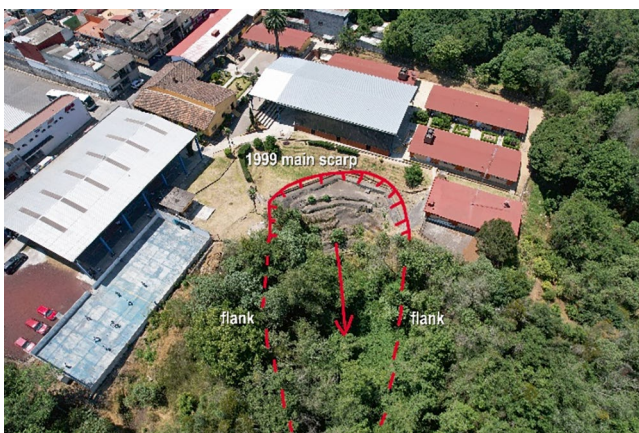
Fig. 11 Shows that “Elvira Cabañez de Flores” school is in a high-risk landslide area in 2023. Drawn lines indicate the main scarp and flanks of the past landslide. (Photo courtesy of Ricardo J. Garnica-Peña)
