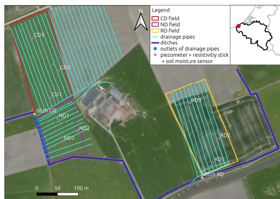
Figure 1. Overview of the experimental site in Middelkerke (Belgium) with three fields equipped (CD, RD and ND). In each field, three locations are monitored (e.g. RD1, RD2, RD3). The drainage system (PVC drains at about 0.9 m depth, spaced 8 m with an average slope of 0.1%) are visible in cyan. In the CD and RD field, the south–north drains are merged into a collector drain and brought to a control pit where an elbow can adjust the water table. Blue dots denote outlet of drainage pipes (or control pit) in the polder-managed ditch (dark blue).
