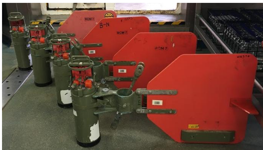
Figure A.5.2. Recording current meter (RCM7) before deployment (Fennell, pers. comm.). The RCM7 is a rotor current meter consisting of a vane to define the flow direction and a recording unit with a rotor (to measure the speed), a magnetic compass and a Fenwall thermistor (temperature sensor). Optional sensors (conductivity and pressure) can be used (Aanderaa Instruments, 2000).
