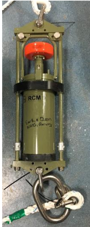
Figure A.5.3. Recording current meter (RCM9) before deployment (Fennell, pers. comm.). The RCM9 consists of a recording unit equipped with an Acoustic Doppler Current Sensor (to measure the speed and direction of the flow) and a Fenwall thermistor (temperature sensor). Optional sensors (conductivity, turbidity, pressure and oxygen) can be used (Aanderaa Instruments, 2001).
