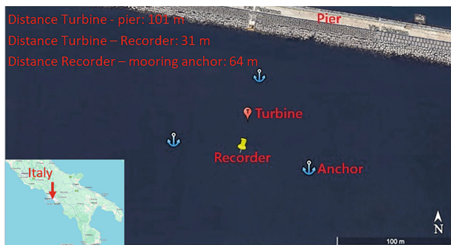
Fig. 1 Positions of the acoustic recorder and distances from the main noise sources. At the top, the Naples harbor pier
