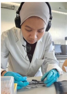
Figure 5. Adjustment of the MinION flow cell position prior to sequencing.
