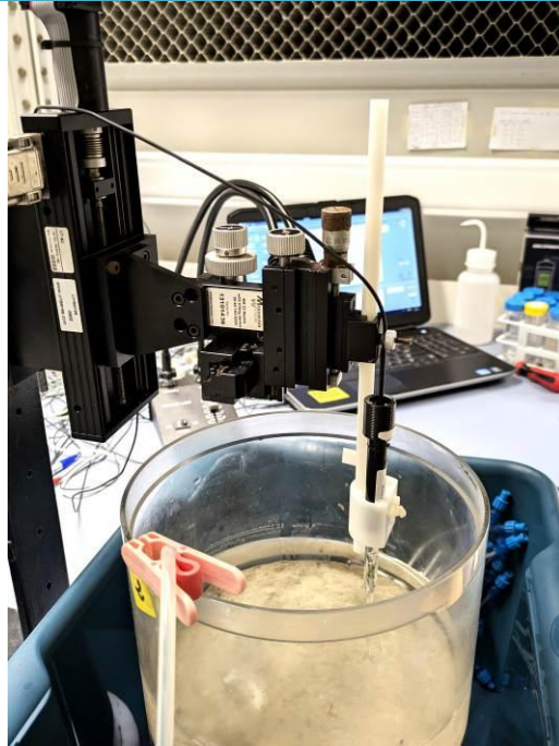
Figure 4: Micro-profiling to detect cable bacteria geochemical imprint
