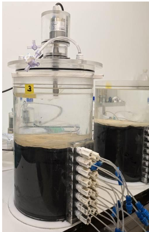
Figure 3: Incubation core setup with Rhizons for porewater extraction
