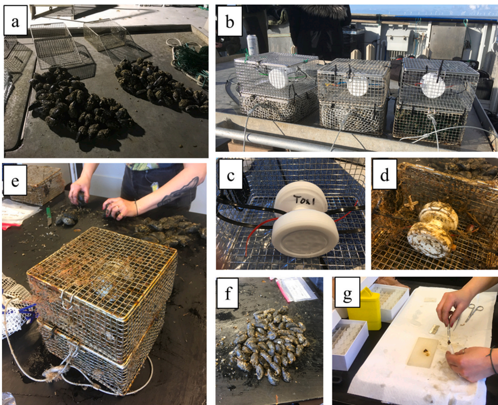
Fig. 5. Photos from deployment (30 March 2022) and recovery (5 July 2022) of mussels and passive samplers at UC30. a) Cages with mussels are prepared onboard RV Aurora. b) Fully packed mussel cages (bottom) and passive sampler cages (top). c) Passive sampler prior to deployment. d) Passive sampler upon retrieval 14 weeks later. e-f) Mussels retrieved from the cages. g) Mussel dissection.
