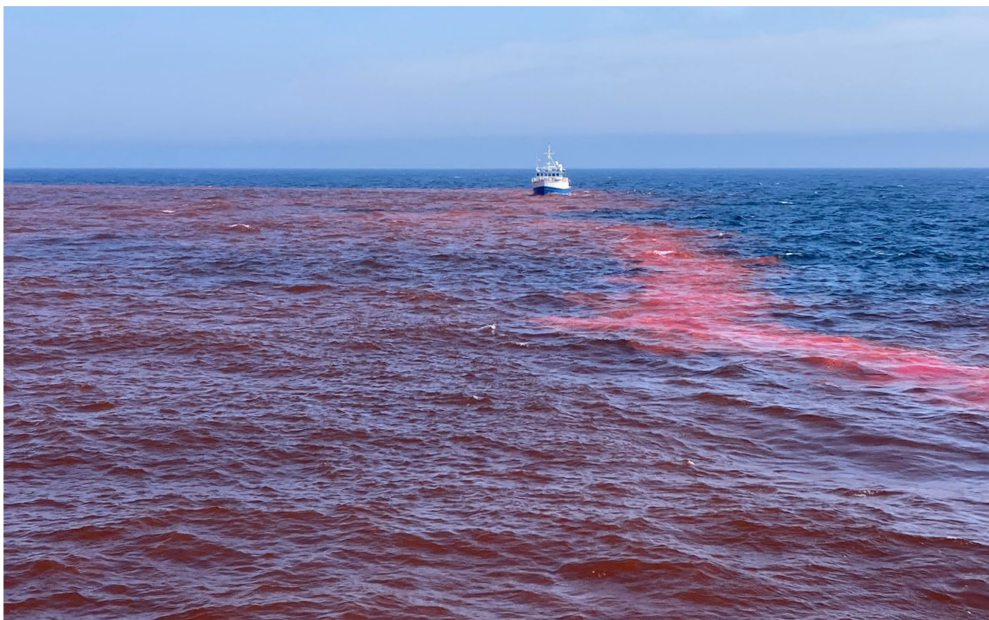
Rhodamine red dye is used in Ocean Alkalinity Enhancement experiments to trace the distribution of added substances.
