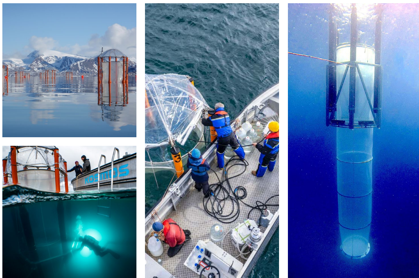
Figure 3.2 Pelagic mesocosm facilities for Ocean Alkalinity Enhancement (OAE) research. OAE increases seawater alkalinity to convert dissolved CO 2 into stable HCO 3 - and CO 3 2- , thus increasing the drawdown of atmospheric CO 2 .
