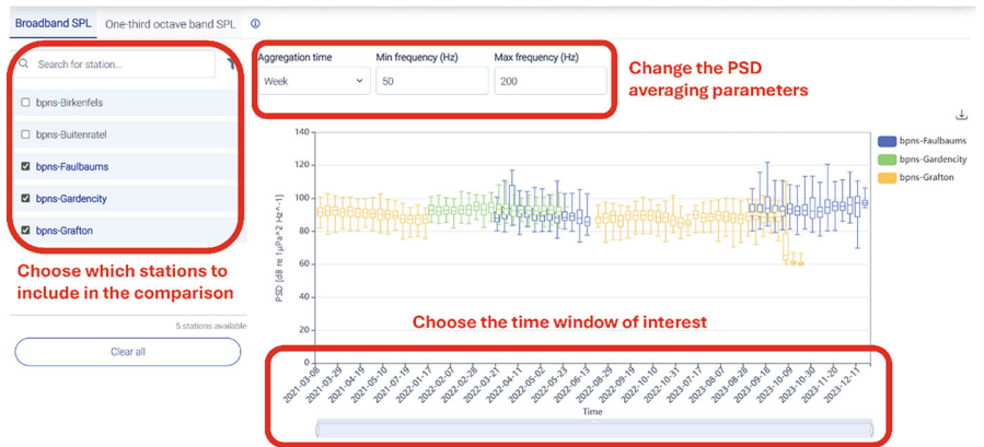
Fig. 5 Compare the sound pressure levels for different stations, represented by different colors, over time for specified frequency ranges
