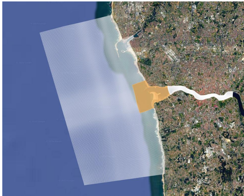
Figure 24. Delft3D decomposed domain showing subdomains for the coastal area, estuary area, and the river area.
