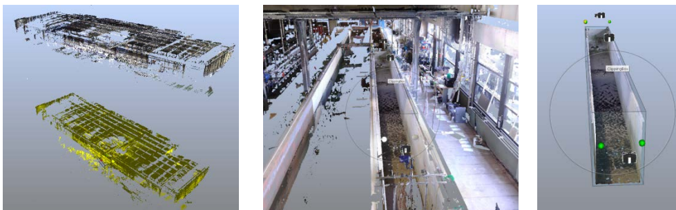
Figure 15: SCENE point cloud matching between scans (center) facility and bounding info (right) applied clipping box to filter for wave flume with dune model only for XYZ point cloud extraction.
