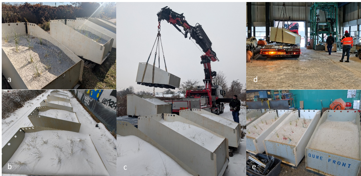
Figure 5: a) DuneCrates November 2025 b) DuneCrates January 2026 with snow cover c) Moving of DuneCrates by boom truck d) Unloading of DuneCrates inside the hydraulics lab e) DuneCrates thawed and with painted vegetation for tracing of plants during erosion experiments
