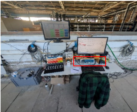
Figure 7: Ultralab HF-58 setup at 1 m wave flume
