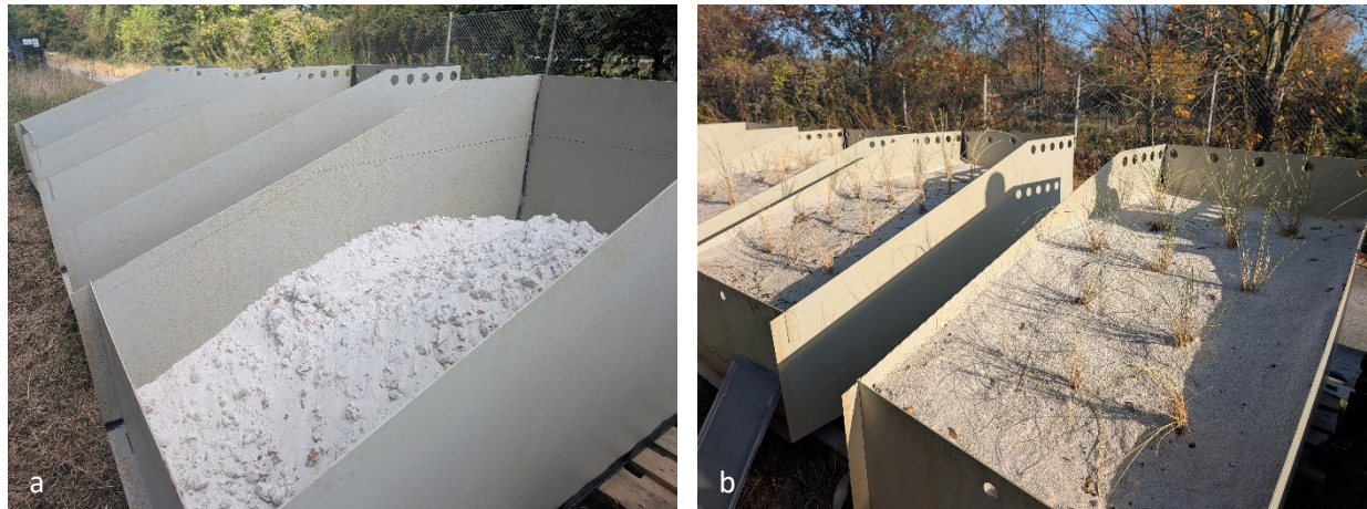
Figure 4: a) Initial setup of the dune crates outside the hydraulic lab with final dune model profile line in black marked b) final stage of top planted DuneCrates
