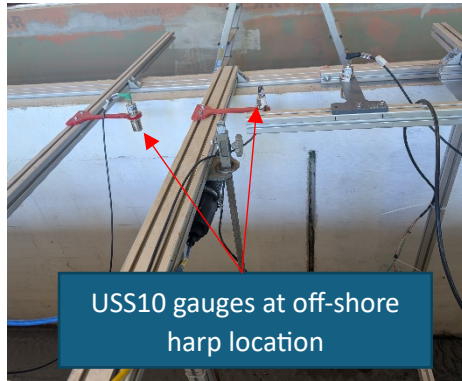
Figure 8: Offshore wave gauge harp in front of data acquisition setup
