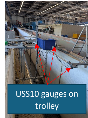
Figure 9: Movable trolley with gauges
