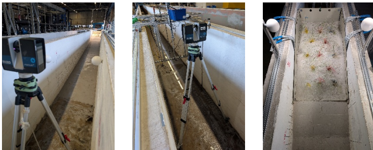
Figure 14: (left) Faro S+ scanner at the dune toe area (center) perspective towards wave maker (right) white reference globes positioned on the instrumentation frame arching across DuneCrate 05.
