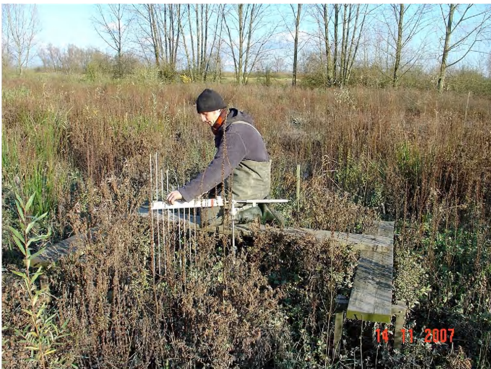
Photo 3. Carrying out SET measurements
