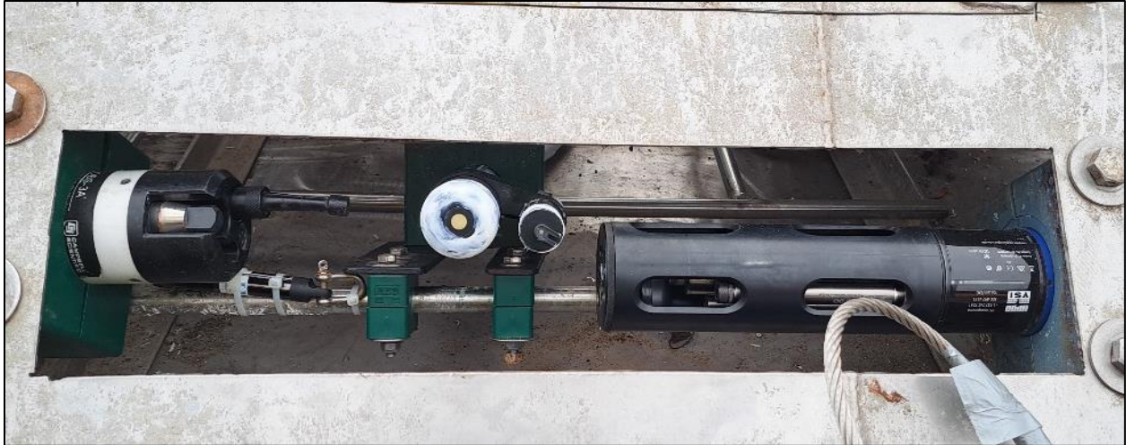
Figure 1. ABS (center) and OBS (right) sensors installed on the bottom frame.
