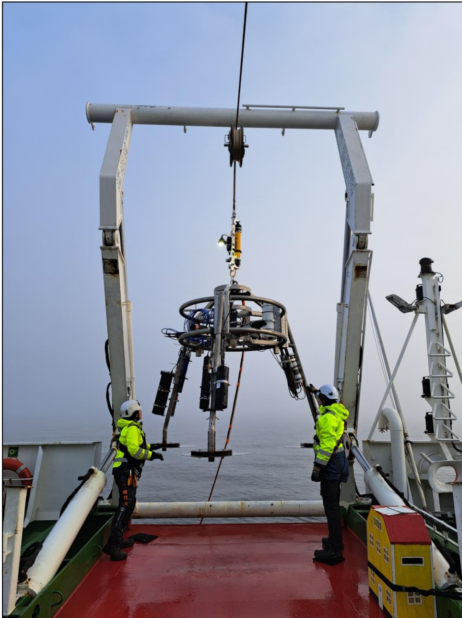
Figure 1. Benthic lander recovered after 7-week deployment. Photo credit: J. Virtasalo.
