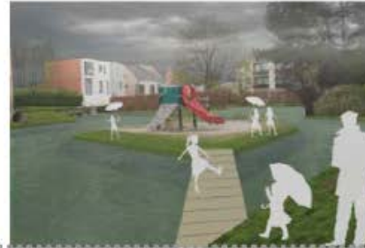
Proposal to convert an existing playground into a multi-use water infiltration/retention facility
