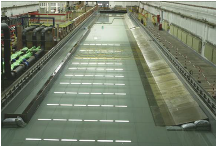
Figure 1: Overview of towing tank with banks
