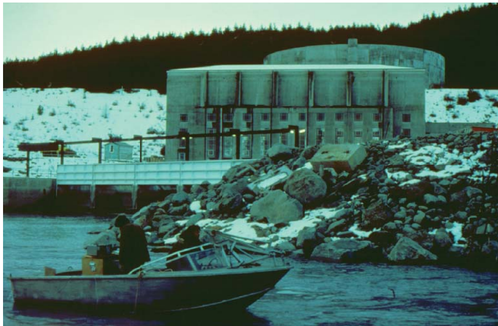
Figure 5.4 | Flow gauging using dye dilution sampling at the upstream end of hydropower canal.
