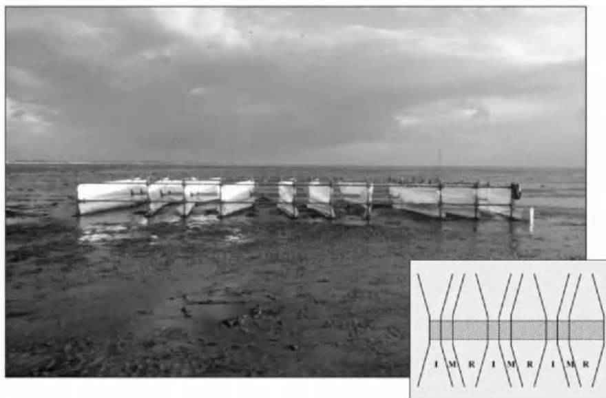
Fig. 3. Front view of the in situ “three-current-flume”, placed in a sheltered seagrass bed and aligned with the prevailing flow direction in a bi-directional intertidal current regime. The flume system (7 m length×12 m width×1 m high) was made of a heavy steel construction with flexible walls of textile awning and consisted of nine lanes. Schematic representation of the flume: by modifying the channel openings the system either increased ( I ), did not notably alter ( M ) or reduced ( R ) the tidal currents in the central section of the flume ( hatched area ) relative to ambient current velocities outside the flume. Each flow treatment consisted of three replicates. The density of Hydrobia ulvae and the biomass of seagrass epiphytes were recorded in the central working section of the flume, as well as in the control areas outside the system
