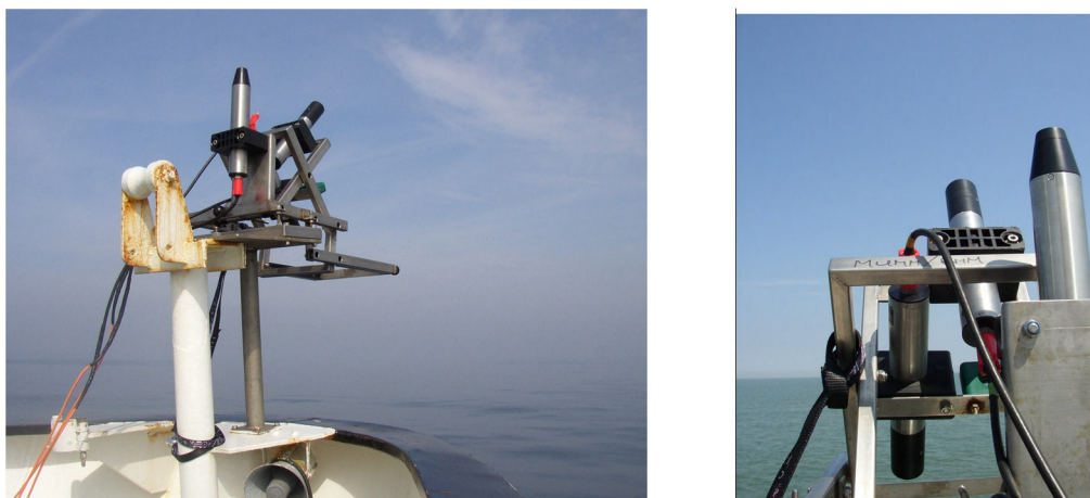
Figure 3: Frame with 3 TriOS-RAMSES hyperspectral spectroradiometers installed on R/V Belgica
