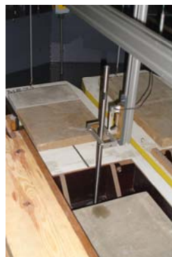
Figure 1: Measuring forces on push-tow combination in scale model
