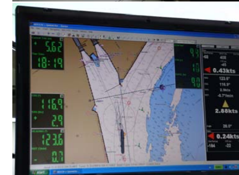
Figure 6. ULCC approaching the Berendrecht Lock, Port of Antwerp, Belgium, assisted by a portable pilot assistance system.
