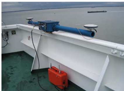
Figure 3: In situ measurement of vessel motion
