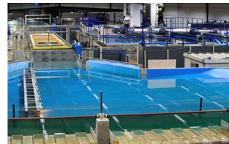
Fig. 2. Hydraulic Model of Post Panamax Locks
