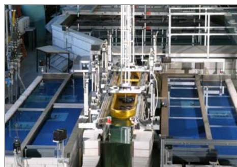
Figure 2: Laboratory model for measuring ship forces in the lock
