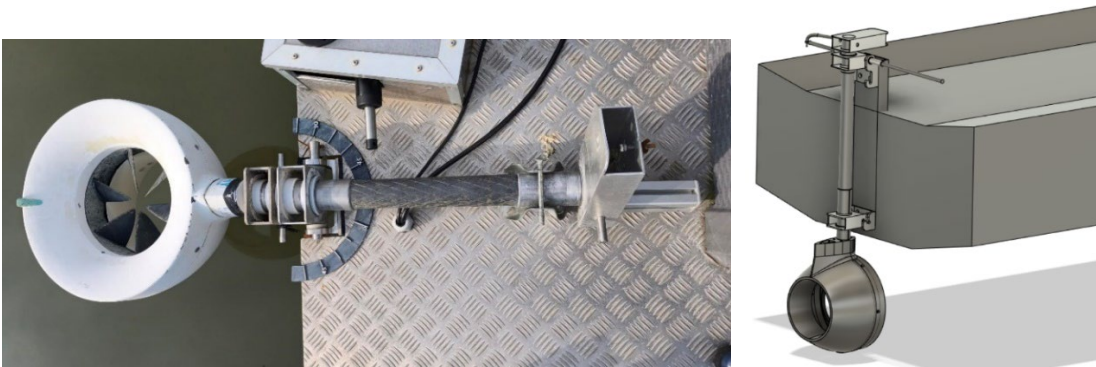
Figure 2. Hy.G Motors, RIM6kW - electric driven thruster lifted on the deck (left) and in operating position (right).
