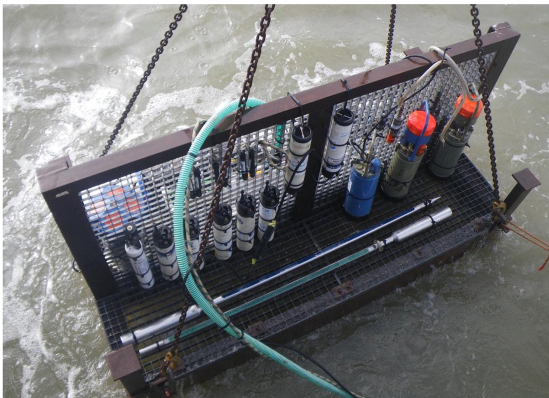
Figure 3-1: Calibration frame with pump set-up
