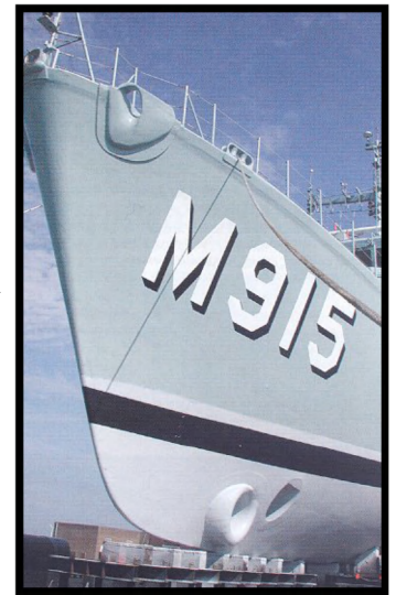
Belgian Navy minesweeper coated with a lining technology incorporating glass platelets into a resin vehicle
