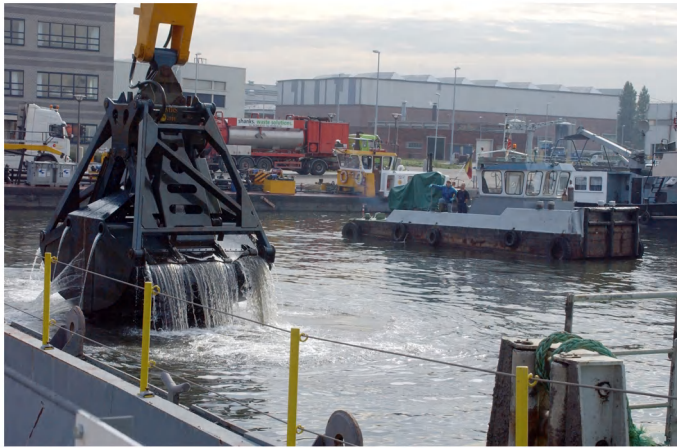
The Antwerp Port Authority's precision grab dredger "The Nose" equipped with valves to minimize resuspension, taking a sediment sample.
