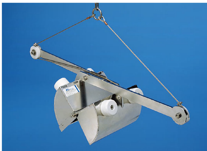
Figure 3. Photograph of a Van Veen grab used for sediment sampling
