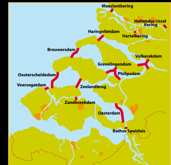
Figure: Levee breach near Papendrecht in 1953 (left page). Locations of the storm surge barriers and dams of the Delta Plan that were constructed in the period between 1958 and 1997 (bottom).
