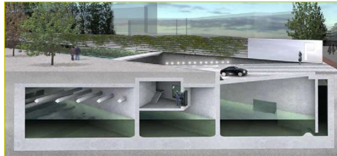
Figure 7.5. Reservoir connected to the sewage and stormwater system being developed as part of a newly built underground parking garage in Rotterdam 36 .
