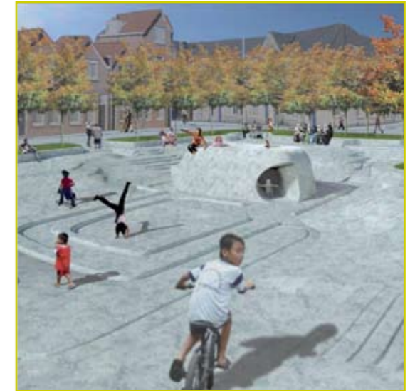
Figure 7.4. Example of a water plaza that is used as a playground during normal conditions and as a reservoir in case of extreme precipitation.
