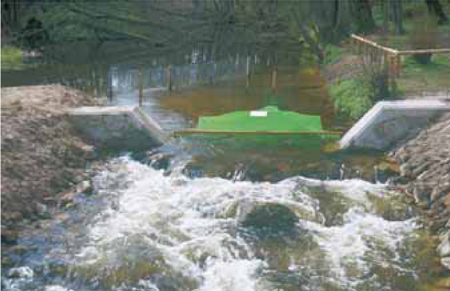
Figure 6.1: Fish trapping to monitor the functioning of the fish ramp at the Pritzhagener Mill on the Stöbber (Brandenburg)
