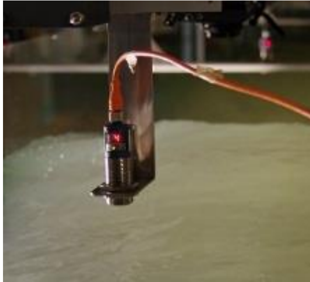
Fig. 2-2 - Mounting of the acoustic displacement meter (ADM) above the channel centreline.
