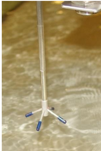
(A) ADV Vectrino II Profiler: photograph (left) and a coordinated sketch (right)
