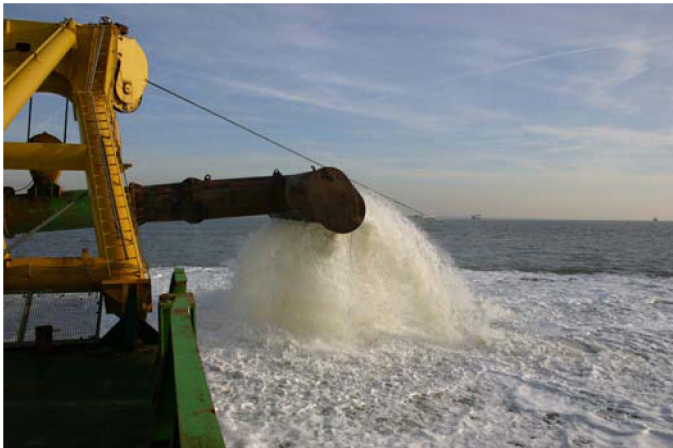
Fig. 10. Detail of the diffuser.
