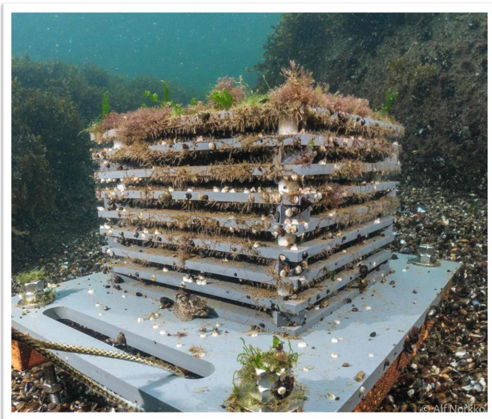
Image: An Autonomous Reef Monitoring Structure (Photo credit: Alf Norkko)
