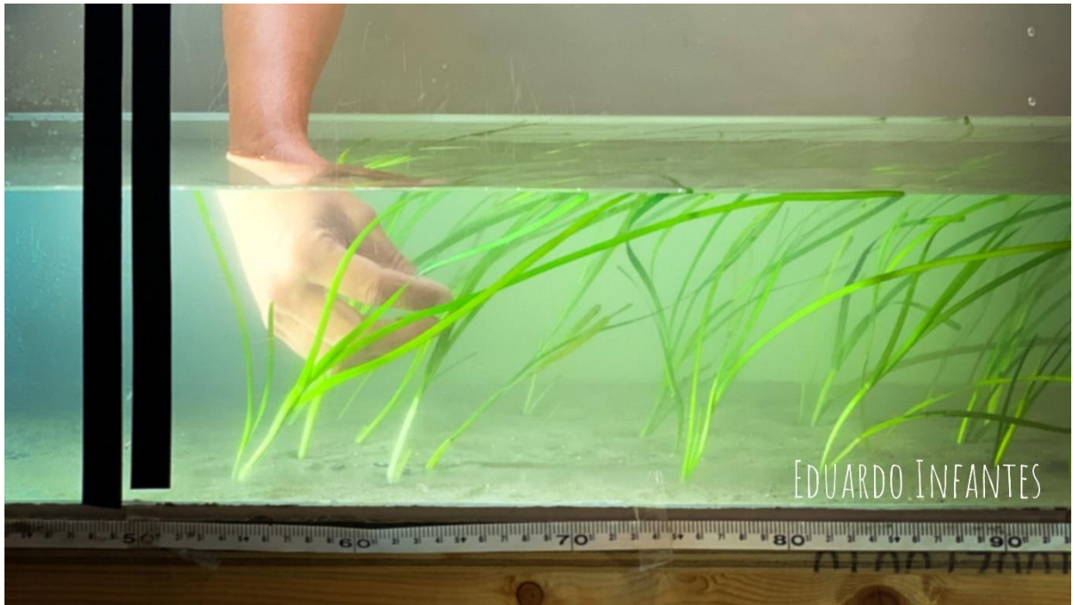
Fig 1 – Seagrass under controlled bio-physical conditions in a hydraulic flume.
