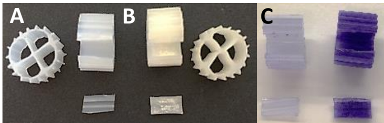
A: fresh beads B: Used beads C: Stained fresh (left) or used (right) beads
