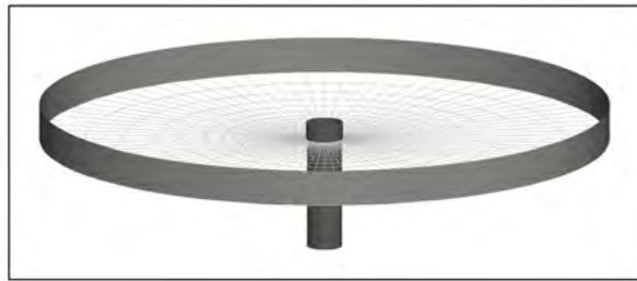
FIG. 5: Computational domain for simulation of circular dropshaft
