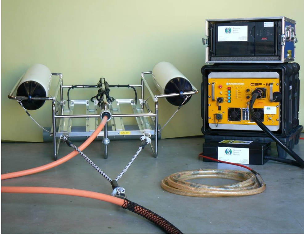
Figure 4 – GSO sparker source (left) and high voltage power supply units(right)
