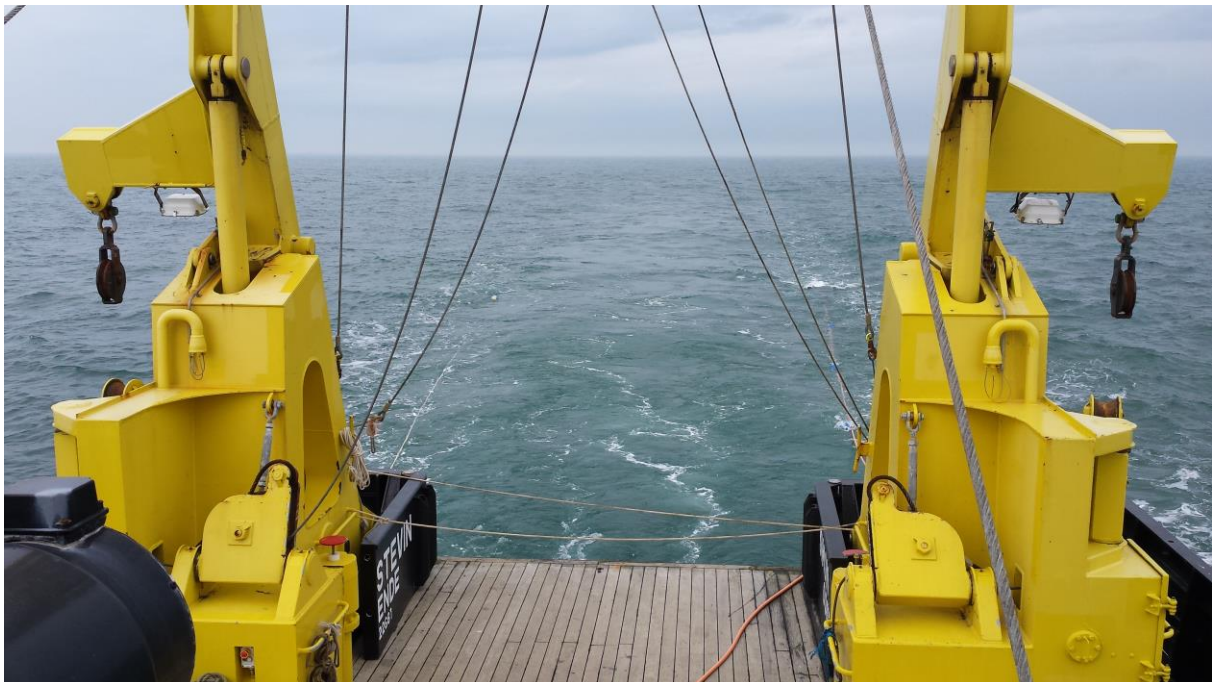
Figure 5 – GSO sparker and SC streamer towed behind the RV Simon Stevin
