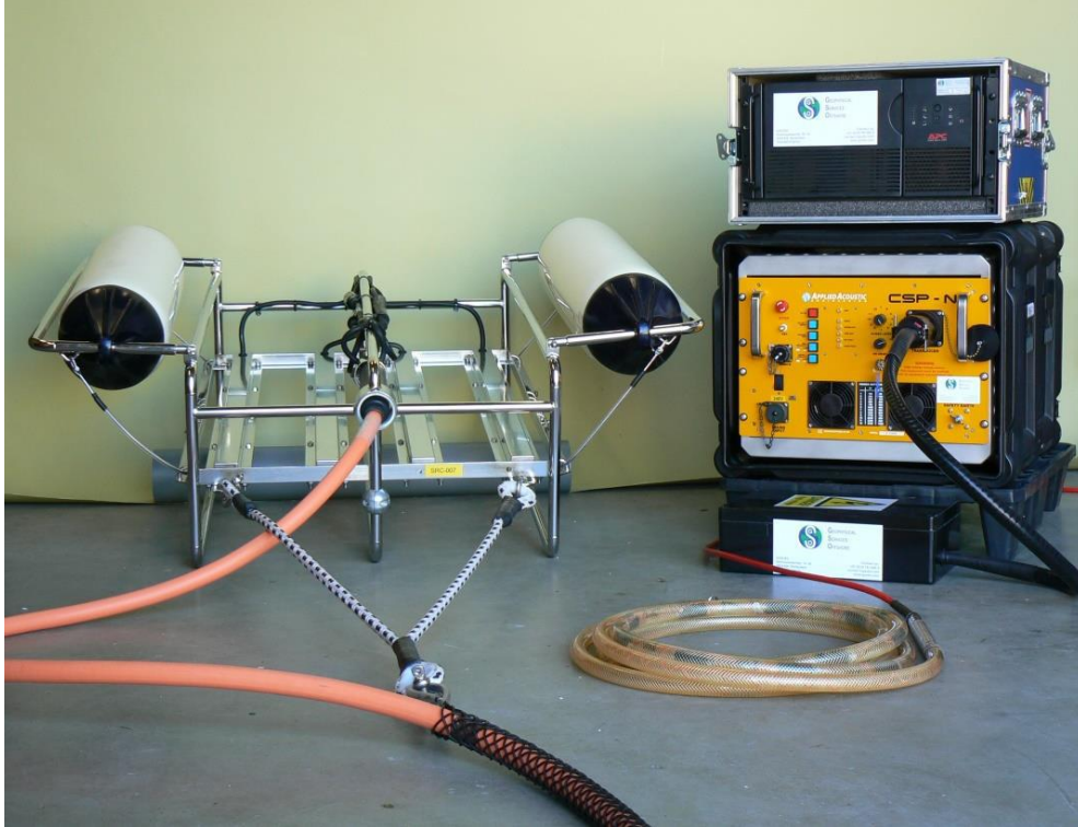
Figure 4 – GSO sparker and High Voltage Power Supply Units
