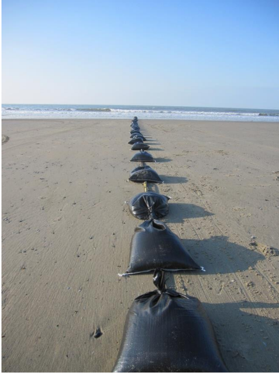
Figure 3 Left: The marine ERT cable on the beach secured with sandbags during low tide on Tuesday. Right: situation on Wednesday after two high tides. The sandbags and cable are partially covered. Viewpoint in the direction of the sea.
