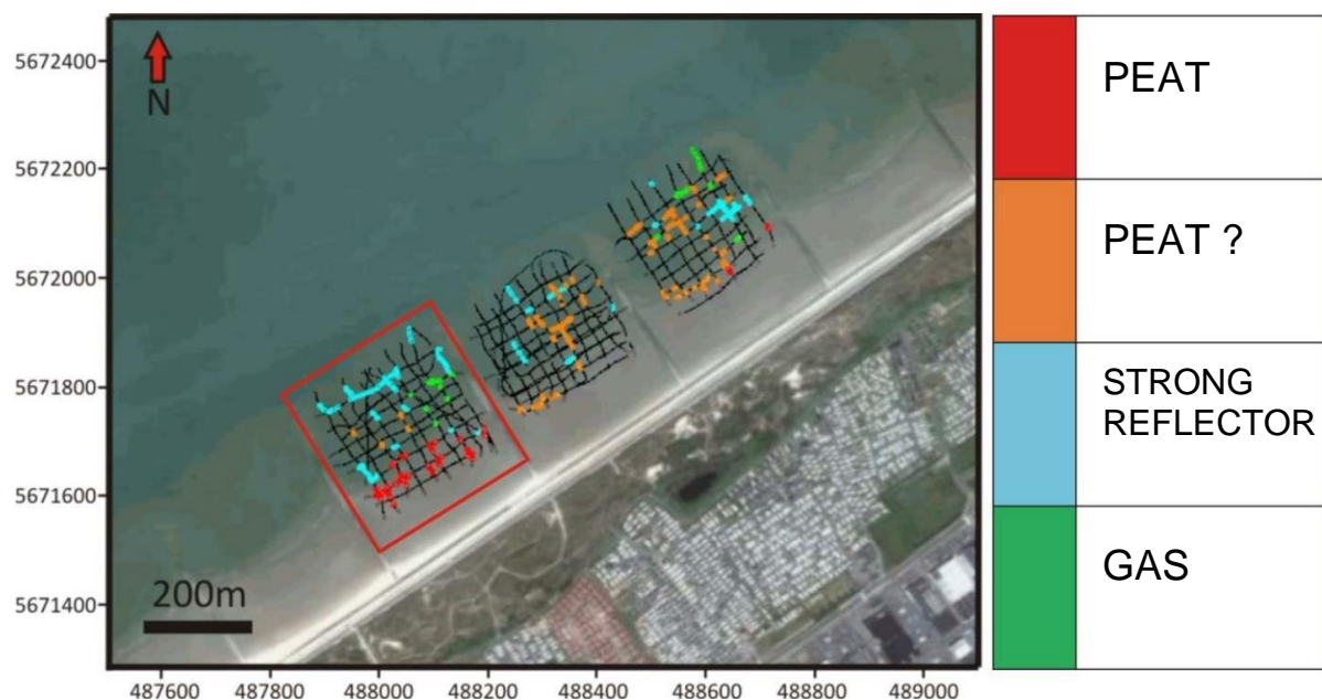
Figure 2. Strong reflectors (blue), the presence of peat (red), suspected presence of peat (orange) and the presence of gas (green). The red rectangle represents the area between breakwaters 22 and 23. Figure from Claerhout, 2014.
