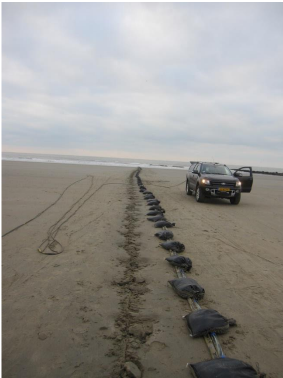
Figure 4 Left: The marine streamers on the beach secured with sandbags during low tide on Wednesday. The location of the marine ERT cable to the left of the streamer is visible by the tracks in the sand. Right: situation on Thursday after two high tides. The streamers are partially covered and the sandbags partially covered or moved. Viewpoint in the direction of the sea.
