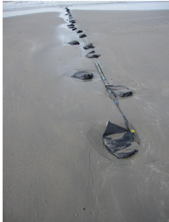
Figure 4 Left: The marine streamers on the beach secured with sandbags during low tide on Wednesday. The location of the marine ERT cable to the left of the streamer is visible by the tracks in the sand. Right: situation on Thursday after two high tides. The streamers are partially covered and the sandbags partially covered or moved. Viewpoint in the direction of the sea.
