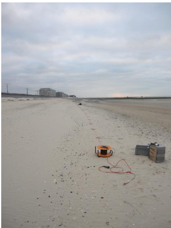
Figure B11 Land ERT on the beach, parallel to the dike (12 October 2016).
