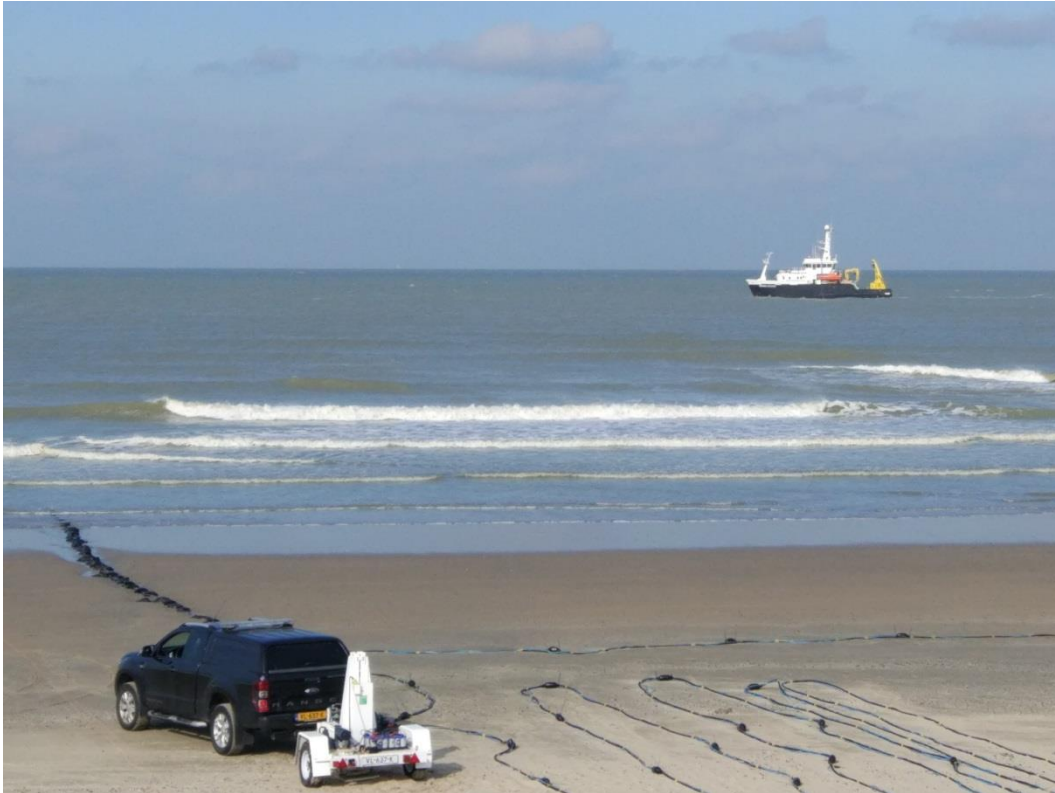
Figure B16 Simon Stevin approaches survey area and returns to Oostende shortly after because the waves are too high. The airtube for the airgun is lying on the beach with floaters attached. The Impactor source (back-up plan) was also ready. 13 October 2016.
