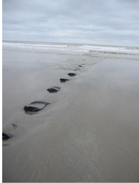
Figure 3 Left: The marine ERT cable on the beach secured with sandbags during low tide on Tuesday. Right: situation on Wednesday after two high tides. The sandbags and cable are partially covered. Viewpoint in the direction of the sea.
