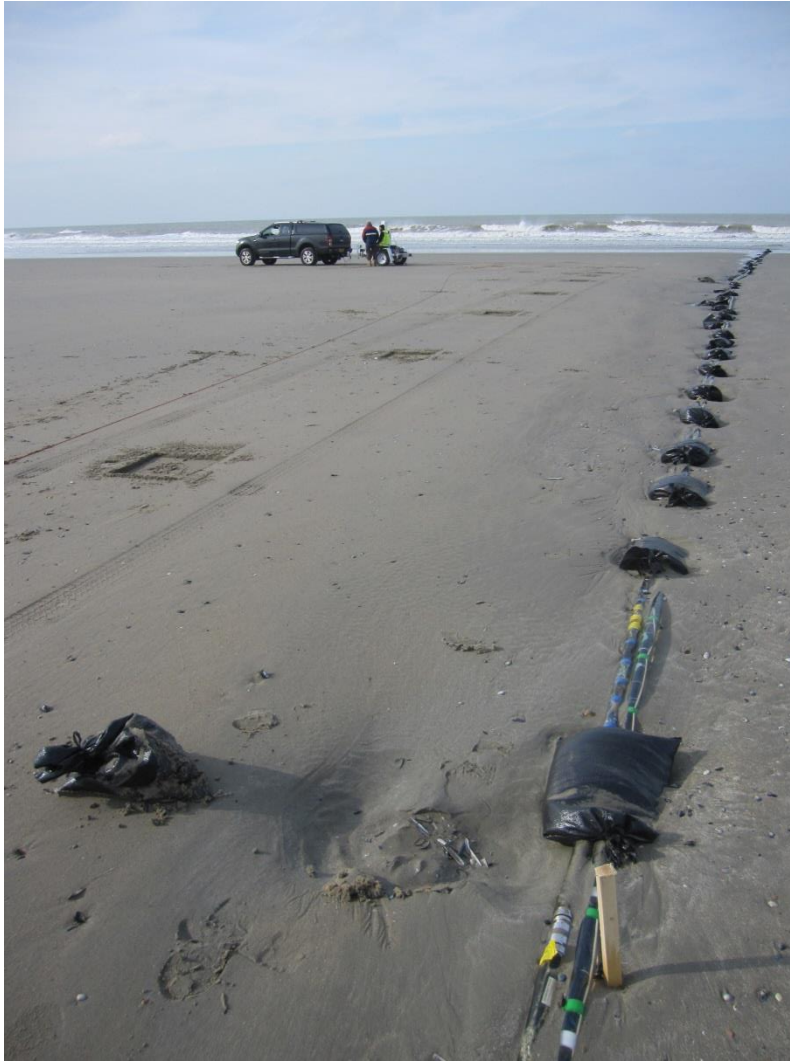
Figure B18 Scholte wave experiment with Impactor source and marine streamer covered by water (13 October 2016). Squares are imprints of shots on the beach.
