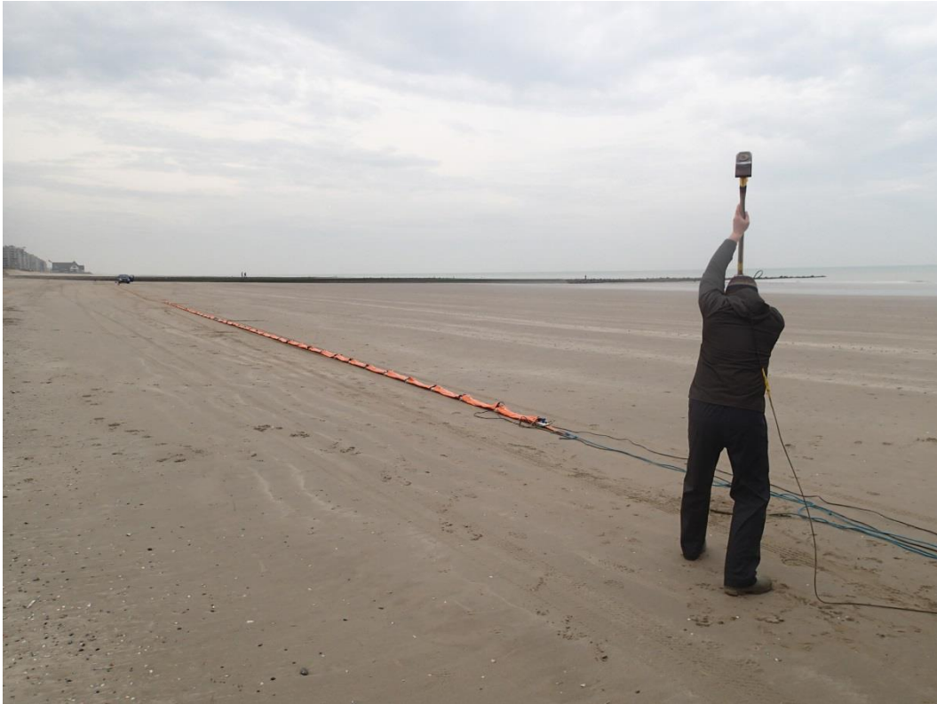
Figure B5 MASW on beach (14 November 2014): hammer blow and land streamer parallel to dike
