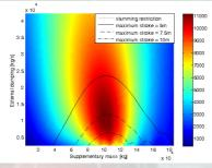
Absorbed power [W] as a function of external damping and supplementary mass with implementation of slamming and stroke limitations for  $\rm H_{s}$  values between 1 and 1.5 m. The buoy is a cone-cylinder with a diameter of 4 m and a draft of 3 m. The area enclosed by the contour lines has to be avoided in order to satisfy the restrictions.
