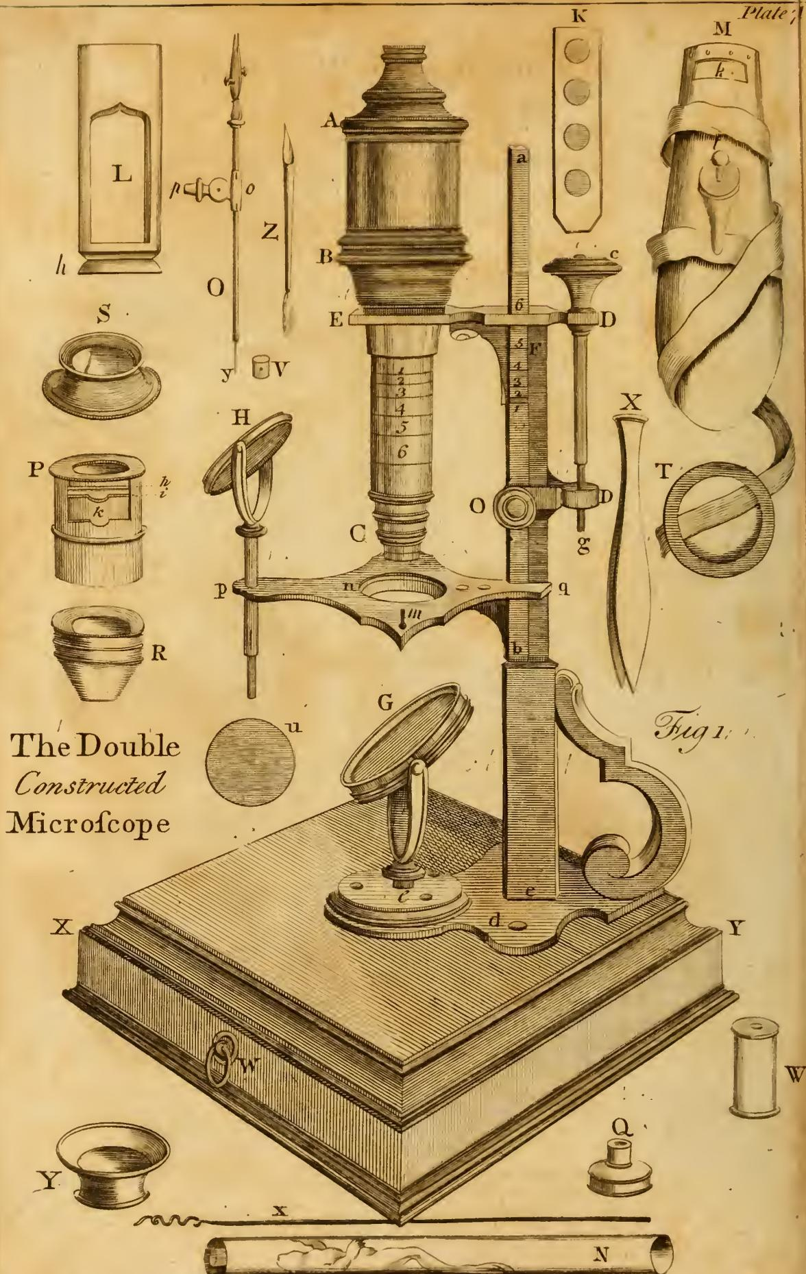
The Double Constructed Microscope
