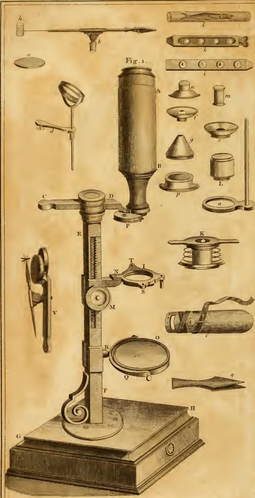
JONES'S IMPROVED COMPOUND MICROSCOPE AND APPARATUS.
